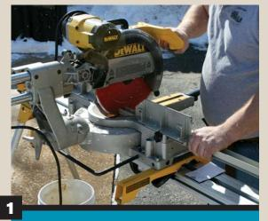
The F-channels, upper and lower tracks, and H-channels — used to join aluminum stormdoor panels together and to framing — are supplied long. Cut them to length using a chop saw; a standard trim blade works well.
